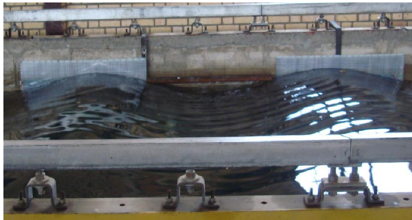
Fig 6) Two horizontal rulers installed over side of the channel.
