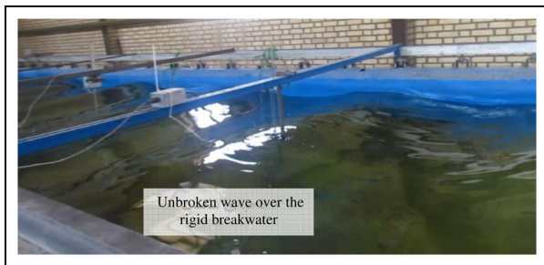
Figure 5. Wave pattern around and over a rigid breakwater, for S = 0.17 , D = 0.1 -R, and h = 0.27 m.
